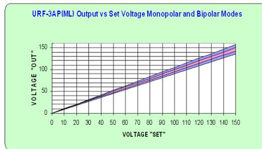
**OUTPUT VS SET VOLTAGE IN MONOPOLAR AND BIPOLAR MODES OVER THE FULL RANGE OF RATED VOLTAGE**
