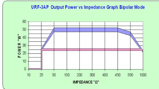
**POWER OUTPUT AT FULL AND HALF OUTPUT CONTROL SETTINGS OVER THE RANGE OF 10 TO 1000Ω**
