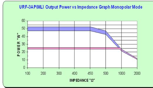
**POWER OUTPUT AT FULL AND HALF OUTPUT CONTROL SETTINGS OVER THE RANGE OF 100 TO 2000Ω**
