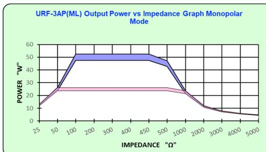
**POWER OUTPUT AT FULL AND HALF OUTPUT CONTROL SETTINGS OVER THE FULL RANGE OF RATED LOAD**
